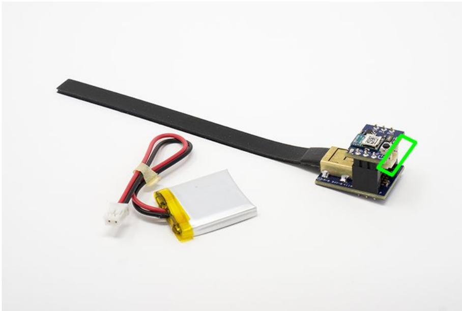
2. Plug the battery into the BLE module. Once plugged into the BLE module it will begin and continue advertising for 30 seconds.
