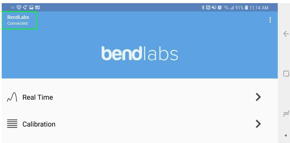
7. Once connected to the device tap the Real Time menu item to see angular output from the connected one or two axis sensor.
